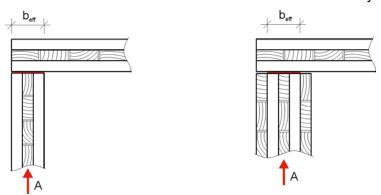
Figure 11: Effective bearing width for determination of contact area
