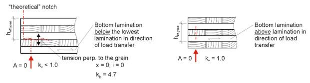
Figure 15: Left – partly supported edge – edge perpendicular to the cover layers Right – partly supported edge – edge parallel to the cover layers
