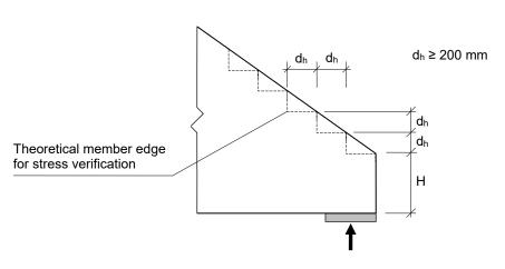
Figure 8: Modelling of an inclined edge by step shaped modelling
