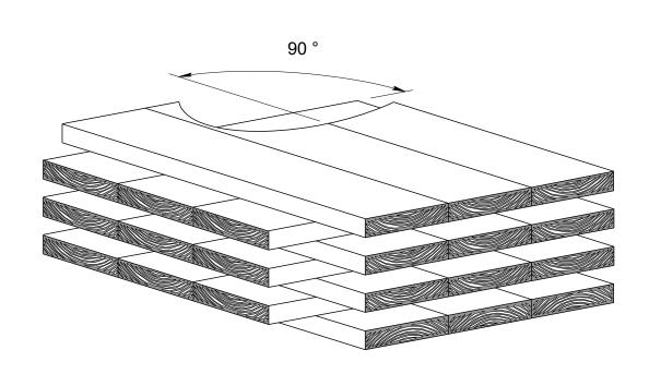
Figure 1: Principle structure of KLH® - CLT
