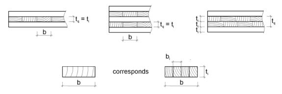
Figure 4: Typical dimensions of cross section of KLH® - CLT lamellas
