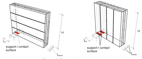
Figure 10: Bearing width and contact area
