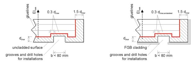
Figure 23: Charring at a groove and at an edge of a wall
