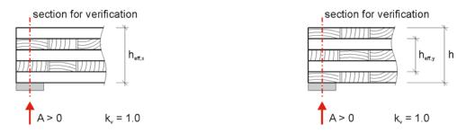
Figure 13: Effective height for calculation of shear stresses
