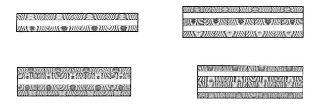
Figure 2: Typical examples of the structure of KLH® - CLT
