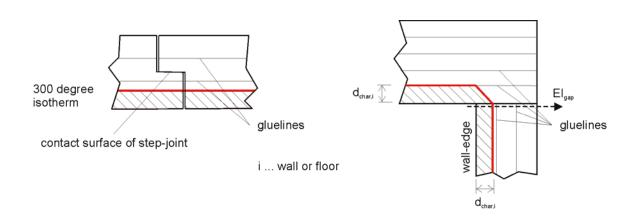
Figure 24: Charring behaviour in the vincinity of a step-joint or an inside corner
