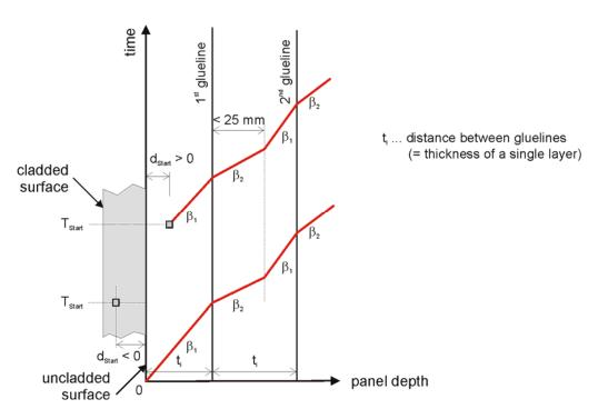
Figure 20: Charring behaviour with and without cladding
