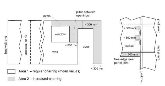
Figure 22: Definition of regions for application of regular and increased charring rates
