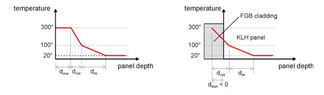
Figure 21: Temperature profiles for non cladded and cladded KLH® - CLT
