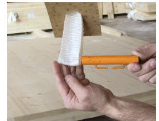
2. Do not position the loop seam in the area of the bolt or lifting hook
