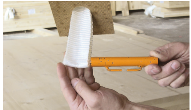
2. Do not position the loop seam in the area of the bolt or lifting hook
